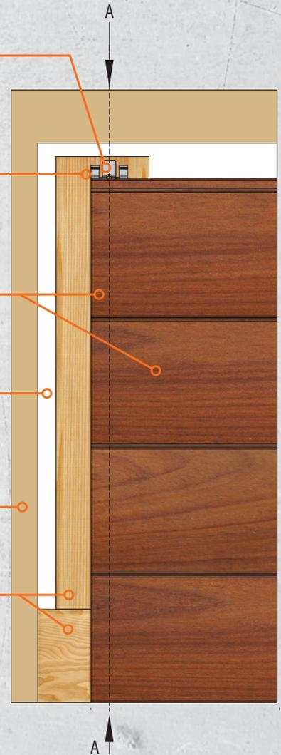
**TIP: Where two pieces of siding butt against each other, use two hidden siding fasteners. (Use two starter clips if there is a butt joint with more than one piece of siding installed on the baseboard).**
