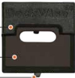
The DeckWise® hardwood deck fixing clip is unlike most “all-metal” fixings which, can react with timber oils triggering staining. The EXTREME® clip is constructed of a hardened plastic polymer resin shell that increases UV & chemical defense qualities; and has a stainless steel insert for reinforcement.
