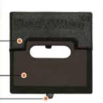
The DeckWise® hardwood deck fixing clip is unlike most "all-metal" fixings which, can react with timber oils triggering staining. The EXTREME® clip is constructed of a hardened plastic polymer resin shell that increases UV & chemical defense qualities; and has a stainless steel insert for reinforcement.
